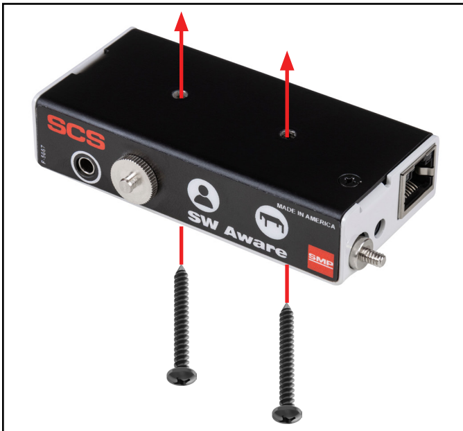
Figure 3. Using the two rounded head screws to mount the SW Aware Monitor
