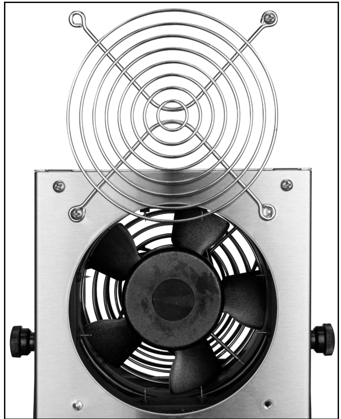
Figure 8. Swinging the rear fan grill to access the emitter pins inside the Ion Pro™ Benchtop Ionizer
