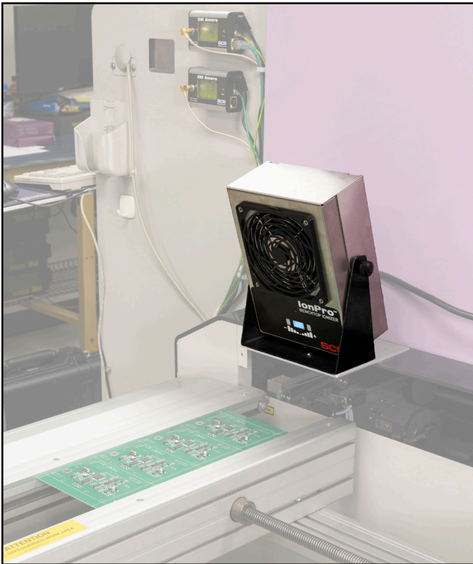
Figure 7. Using the Ion Pro™ Benchtop Ionizer at a machine station
