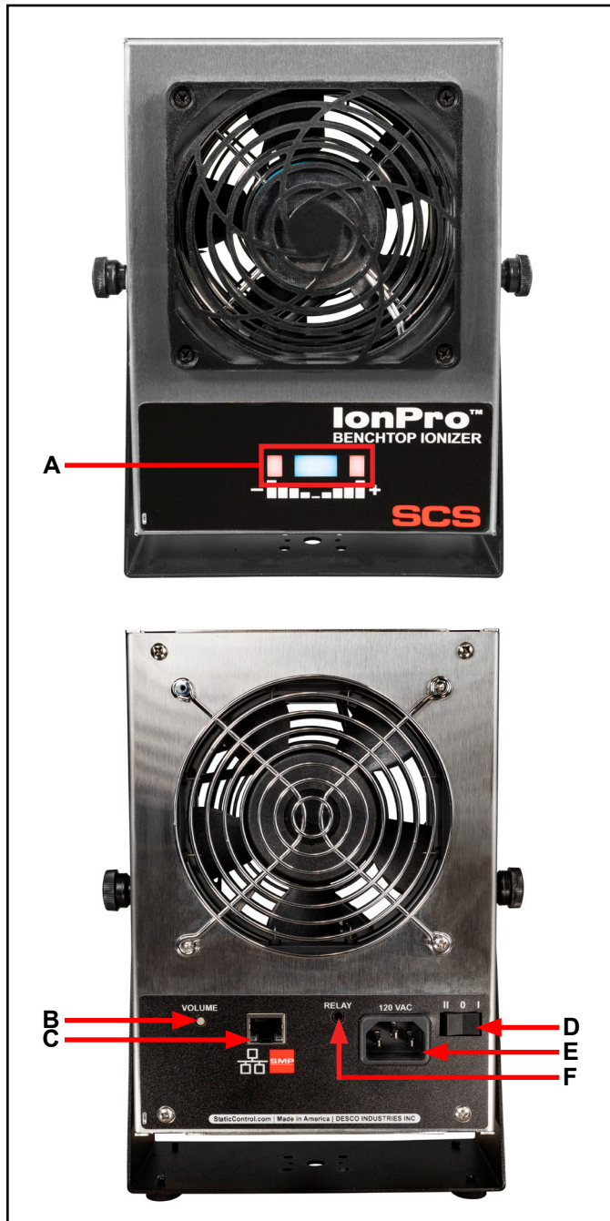
Figure 2. Ion Pro™ Benchtop Ionizer features and components
