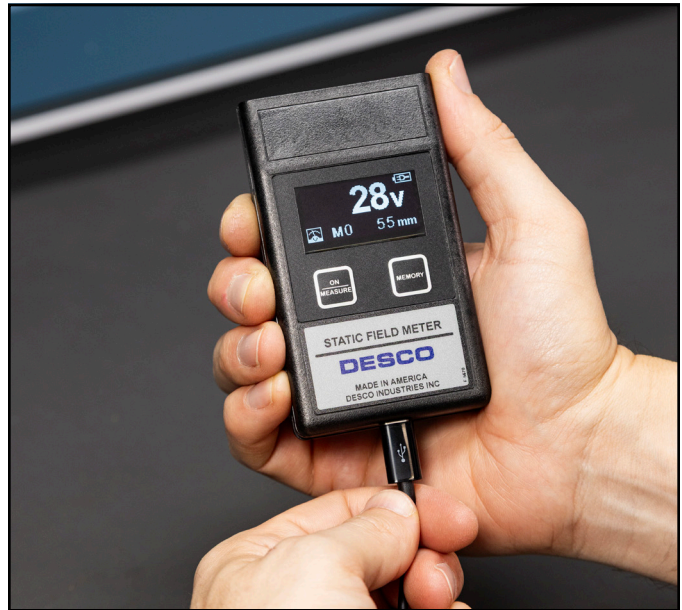
Figure 8. Connecting the USB-C cable to the Static Field Meter
