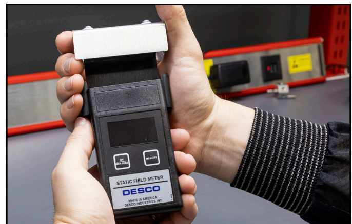
Figure 13. Sliding the Conductive Plate onto the Static Field Meter
