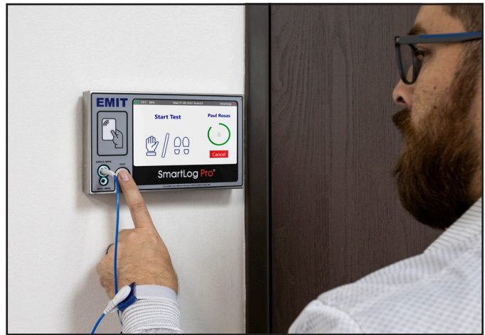
Figure 26. Performing a single-wire wrist strap test
